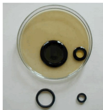
Figure 15. Effect of higher contents of FAME in aviation fuel on volume of rubber in long-term storage [97].
